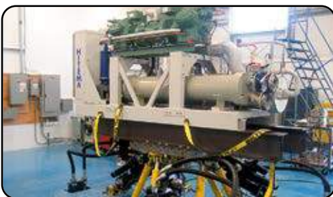
* Seismic test, installed in Canada, 300 kW
