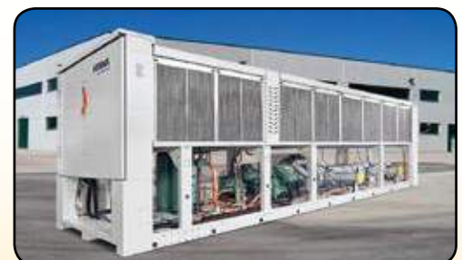
Freecooling liquid chiller with double refrigerating circuit, double hydraulic circuit and double power supply installed in Russia. 522kW @ +3°C LWT
